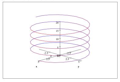
radius of curvature:  $r(t) = \frac{1}{\kappa(t)} = \frac{1}{\frac{45}{229}} = \frac{229}{45}$  at each point.
