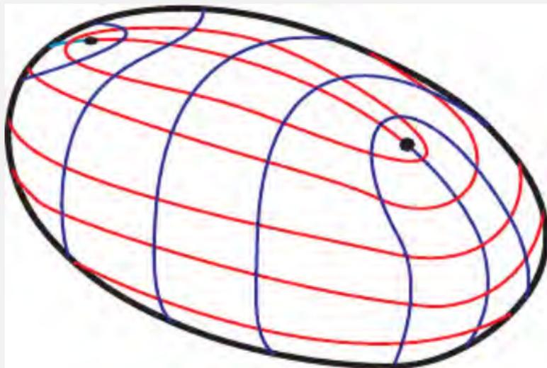
Lines of curvature and umbilic points on a triaxial ellipsoid.
