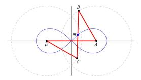
In this picture, AD = BC = 2,  $AB = CD = \sqrt{2}$ , A, D are fixed, and B, C rotate freely about their respective circles. The midpoint m of BC traces out the lemniscate shown above.
